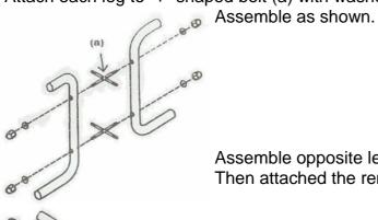
Assemble opposite legs to the "+" shaped bolt. Then attached the remaining legs.
