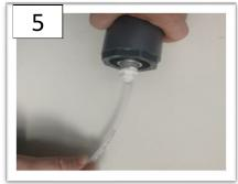
Route the Water Line from Reservoir to Bottom of the Unit. Insert and Push ¼" Tube into the Bottom Fitting.
