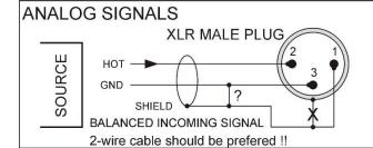
Unbalanced Cable (Signal) to Balanced Input
