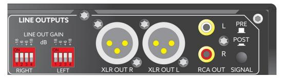
The "SIGNAL" switch is located on the back panel in the "LINE OUTPUTS" field.
