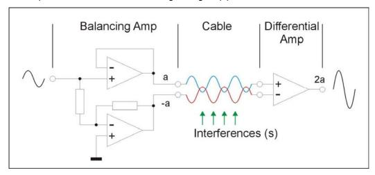
In the receiving device, the balanced signal is processed by a differential amplifier which detects the difference between both:
