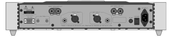
The rear panel will look similar to Figure 1 (above). Each channel has one balanced (differential) input on an XLR connector and one unbalanced (single-ended) input on a RCA connector. There is no switch to toggle from balanced mode to single-ended mode. You may operate the amplifier in either mode, but only one mode at one time for each channel.
