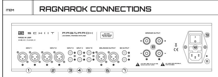
**1 Balanced Input.** This is one of two balanced inputs on Ragnarok. Connect any balanced source here with high-quality XLR cables. 2 Another Balanced Input. This is another balanced input, just like the first one, except it's labeled "Input 2." **3 Single-Ended Input.** This is one of three single-ended inputs. Connect any singleended input here. 4 Another Single-Ended Input. Just like the first, except for the label.
