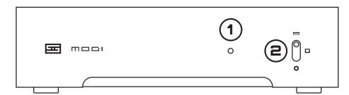
**1 Power LED.** This lights up when you have Modi 3 plugged into a computer, or into an external power source. It doesn't signal UFOs or anything.
