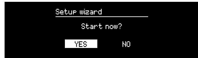
To start the setup wizard, rotate the **CONTROL KNOB** to highlight **YES** and then press the knob to **SELECT**. If you choose **NO**, your R5 will start without configuring time/date and network settings.
