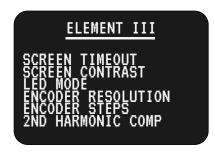
Pressing down on the Volume Knob for 3+ seconds enters the Options Menu. Turn the knob to navigate up/down the options menu Push the knoh to make a selection
