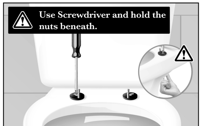
4. Firmly tighten using screwdriver while holding wingnuts.
