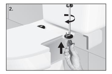
**3. Attach seat, adjust, and tighten screws** <u>very firmly</u>**.** (It may be necessary to hold wing nut to keep it from turning.)
