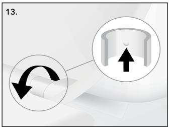
**Note:** Store child seat for future use. To re-install, simply remove C-rings and snap child seat into place.
