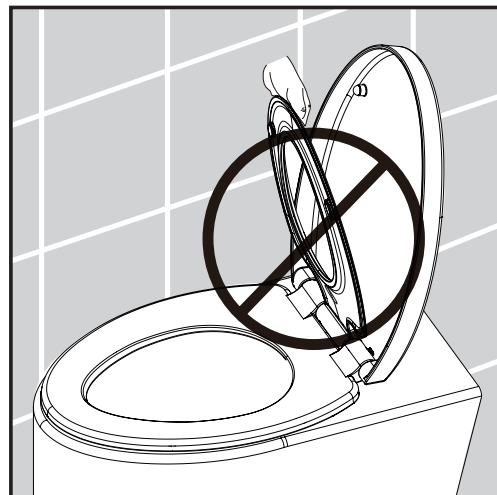
Note: Child seat must be held at 45 \pm 5^\circ , to install or release.
