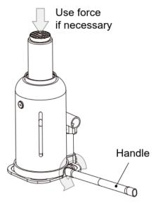
7. Turn release valve (R7) clockwise to the closed position and check for proper pump action. It may be necessary to perform the above step more than once to assume air is evacuated totally.
