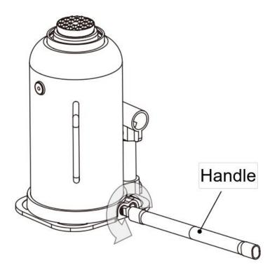
2. Pump handle 6 to 8 full strokes. Leave handle in down position to expose oil fill plug.
