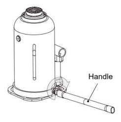
8. Secure the handle in place inside the handle socket. Without any weight on the jack. Cycle the lift up and down several times to insure the hydraulic system is operating properly. (Perform to the Air Purge Procedure again if neccesary.)
