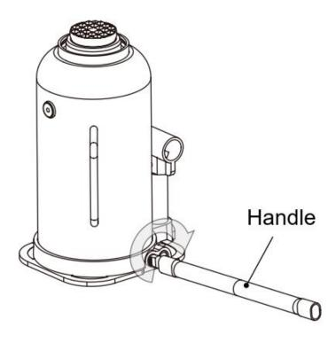
4. Pump handle until the ram reaches maximum height and continue to pump several times to remove trapped air in the ram.
