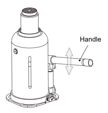
3. Turn release valve clockwise to the closed position.
