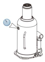
6. Turn release valve counterclockwise to the open position one full turn and lower ram to the lowest position.
