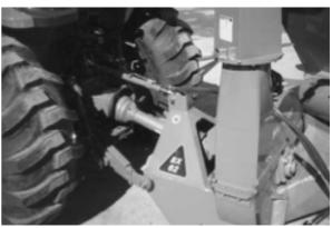
Do not place metal, bottles, cans, rocks, glass or other solid material into the wood chipper. If something like this gets into the machine, stop the machine immediately for a detailed inspection. Stop engine, remove ignition key and place in your pocket and wait for all moving parts to stop before inspecting or unplugging. Inspect machine for damaged or loosened parts before resuming work.
