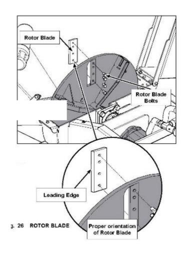
recommended that the clearance between the rotor and stationary blades be set and maintained at 1/32 to 1/16 " (.76 - 1.52 mm) to obtain the best performance.
