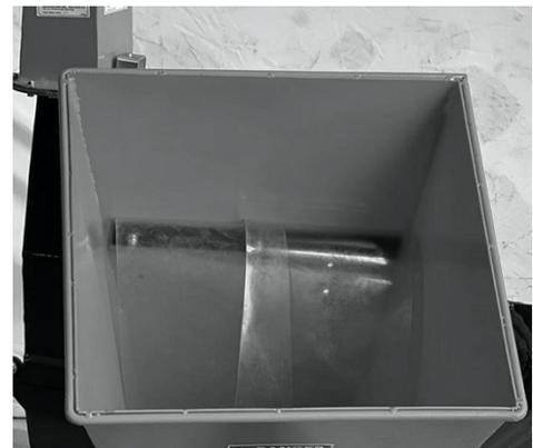
6. Check the condition of the curtain in the feed hopper. It must be in good condition to prevent chips from flying out.
