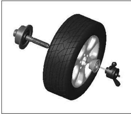
Main shaft-wheel— suitable cone (small head towards inside)—quick handle nut
