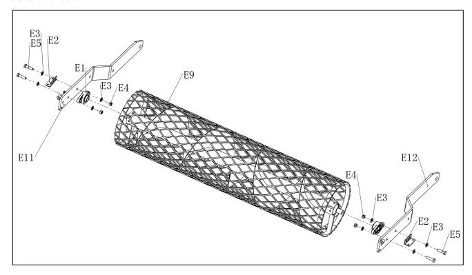
2. When the scraper welding parts installed (E10), it is necessary to place the welding parts of the left and right connecting arms (E11,E12)of the mesh wheel at the same height, then fasten them with bolts(E8), washer(E6), lock nut(E7), and then install the tension spring(E17) according to the below figure.
