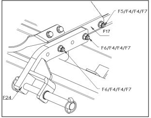
**Note:** Paying attention to the different bolt lengths of the hanging weldment and the hanging assembly under tightening extension (F6 and F5),
