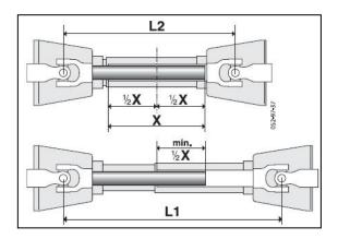
The minimum overlap of inner and outer coupling tube 1/2X size should be 220mm, if the size less than 100mm, please change the coupling
