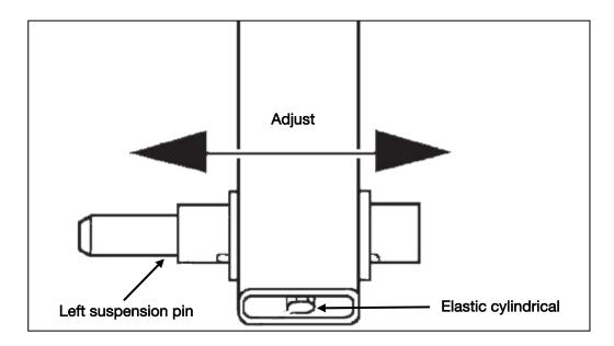
d. Adjust angle, to obtain the most appropriate cutting angle, adjust the upon 3-point linkage suspension to ensure the suitable cutting angle.
