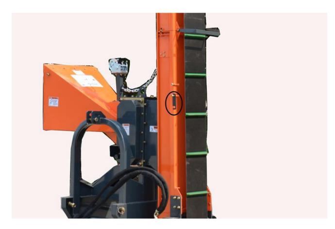
Step 2: Loose winch, lay conveyor on ground and tight bolts on both sides
