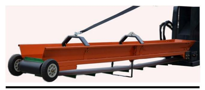
**STEP 3: Turn winch and adjust conveyor to proper angle**
