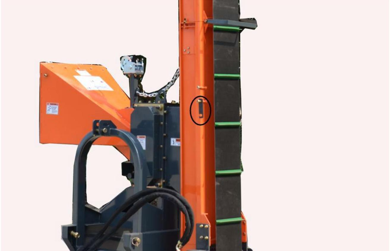
**Step 2: Loose winch, lay conveyor on ground and tight bolts on both sides**
