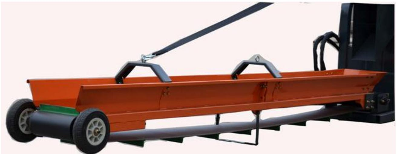
**STEP 3: Turn winch and adjust conveyor to proper angle**
