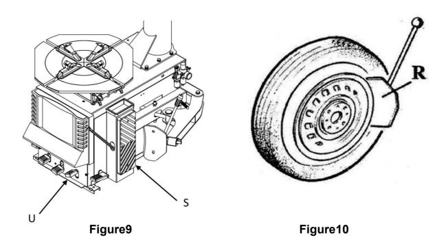
♦ As shown in Figure 10, make the pressing-tire spade R close to the rim edge for
