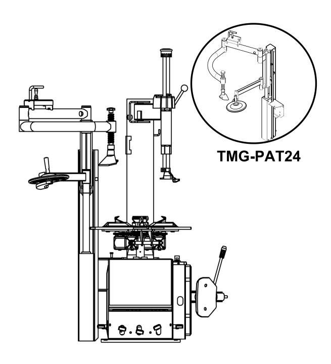
Pneumatic Assist Arm (**TMG-PAT24**) include TIRE-PRESSING BLOCK, TIRE-LIFTING DISC, it can easily dismount Run-flat and Low-profile tires, practical and saving space
