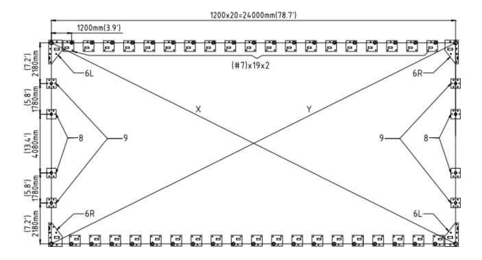
· Installation diagram of expansion bolt.
