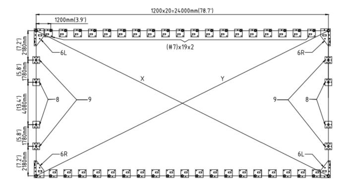
Installation diagram of expansion bolt.
