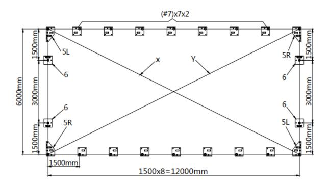
• Installation diagram of expansion bolt.
