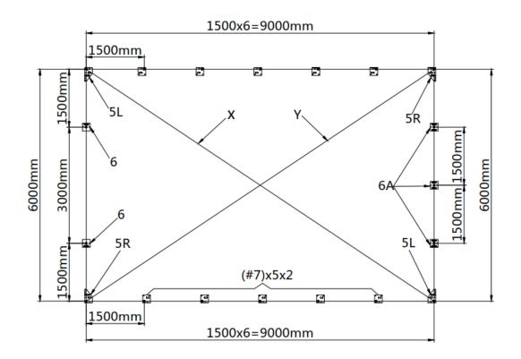
• Installation diagram of expansion bolt.
