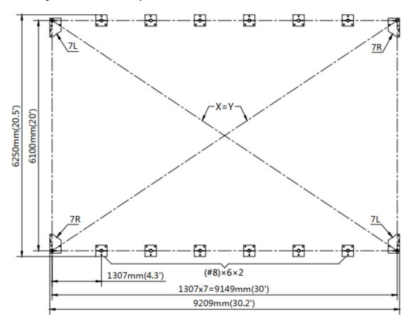
• Installation diagram of expansion bolt.
