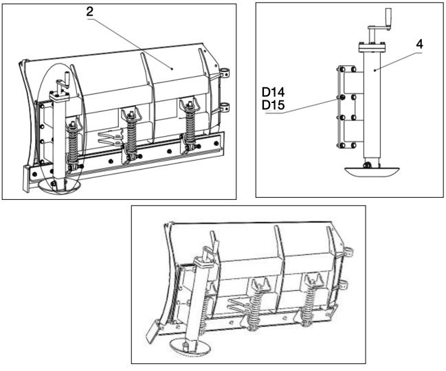
**Installation steps:** Fasten the support adjustment component to the left main shovel with M12\*30 bolts (D15) according to the position in the above figure.
