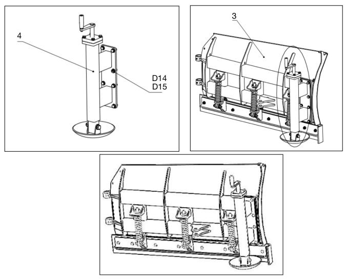
**Installation steps:** Fasten the support adjustment component to the right main shovel with M12\*30 bolts (D15) according to the position in the above figure.
