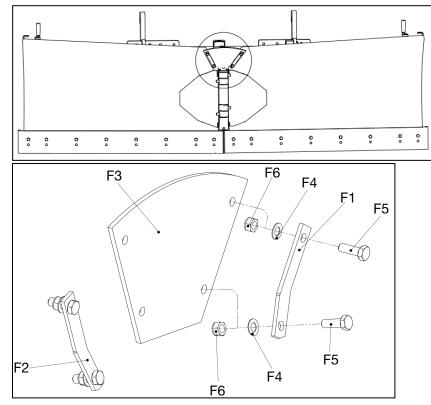
**Installation steps:** Assemble the eraser in the order of the style above. **Importance:** All bolts are locked in place without shaking.
