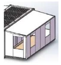
11. Use L-shape corner covering to fix Wall-A & Wall-C /Wall-1 & Wall-3.
