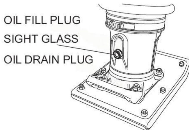
Figure 13 Foot Housing Drain Plug
