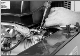
PLEASE NOTE\*\*\*The idler screw needs to be wound fully out failure to do this will result in the engine not running at its full RPMs' which will result a poor cut.
