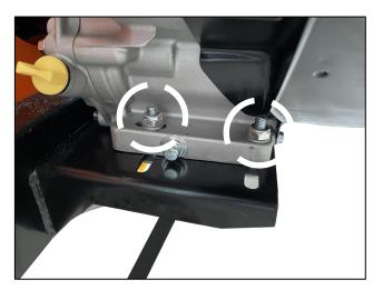
To tighten the drive belt, start by loosening the four bolts that secure the engine to the engine mount using a 16mm wrench.
