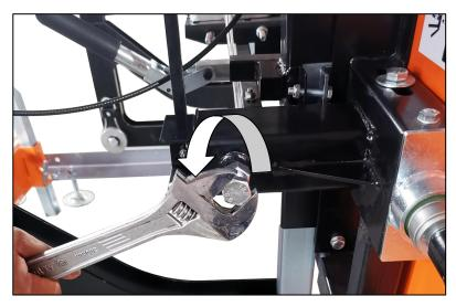
Loosen the tracking alignment locking nut with an adjustable wrench.
