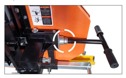
\*Note – It is very important to take the tension off of the blade by turning the "T" handle in the counter-clockwise direction when the sawmill is not in use. Failure to do so, will result in flat spots on the rubber belts. These flat spots will cause the mill to vibrate excessively during next use.\*
