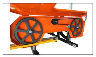
Remove the tension in the blade by turning the "T" handle in the counter-clockwise direction and then open the blade guard cover. The blade should now be loose and free to pull straight out the front.
