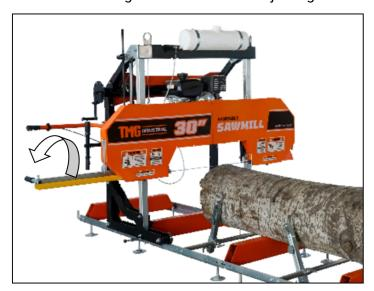
Take some tension off of the blade by turning the "T" handle in the counter-clockwise direction one full turn from full tension position.
