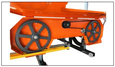
Remove the tension in the blade by turning the "T" handle in the counter-clockwise direction and then open the blade guard cover. The blade should now be loose and free to pull straight out the front. The new blade can now be installed, guards closed and proper blade tension set.
