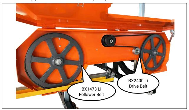
There are two rubber "V" belts on the sawmill and they should be replaced as a set. It is not advised to replace individual belts separately. It is recommended to use a BX2400 Li drive belt for the drive side and a BX473 Li follower belt.
