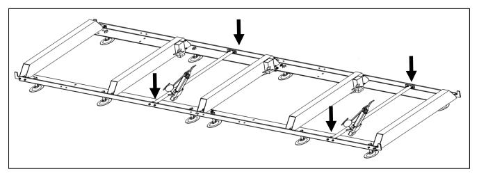
Insert log supports into track cross supports and secure with "T" handles. The "T" handle threads should be coated with waterproof grease. The sawmill includes two sets of log supports – a short set and a long set. The longer set is ideal for larger logs and the shorter set is ideal for small logs and square cants.
