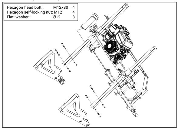
5. Assemble rear vertical post to wheel assembly using the two bolts and back plate. Repeat same step for the other rear vertical post assembly.
