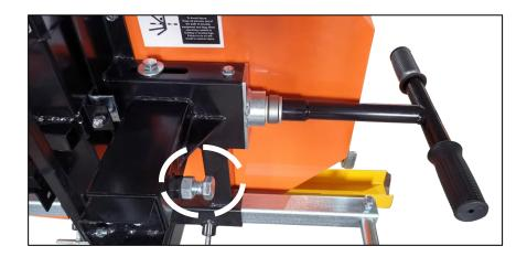
When tensioning the blade, make sure the tracking adjustment bolt sitting behind the T handle (pictured) is sitting back in its recess after you have finished and *before* the mill is run. Failure to do this will result in the blade being thrown and possibly broken.
