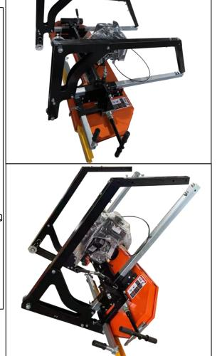
8.Slide the cross beam into the two square tube post. Bolt the top of the square tube post and the cross beam
