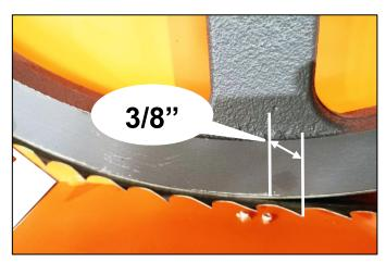
Re-tension the blade by turning the "T" handle a full turn in the clockwise direction. Wearing gloves, spin the bandwheel with your hand and observe how the blade has changed tracking.
