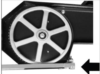
Ensure the blade support arm is locked into place after tensioning the blade.
