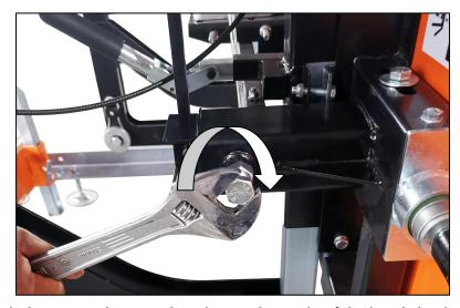
The alignment bolt can now be turned to change the angle of the bandwheel and track the blade. To move the blade more rearward on the bandwheel, this bolt will need to be turned clockwise. Alternatively, turning the bolt in the counter-clockwise direction would force the blade to run more forward on the bandwheel. Turn the bolt a 1/2 turn and re-tension the blade.
