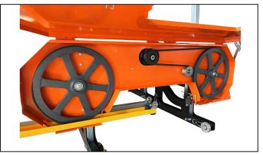
Remove the tension in the blade by turning the "T" handle in the counter-clockwise direction and then open the blade guard cover. The blade should now be loose and free to pull straight out the front.
