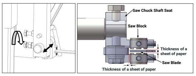
Loosen the blade guide assembly bolt with a 16mm socket. The round shaft should now be free to slide back and forth. Position it so that there is a paper width gap between the bearing and the back of blade. Tighten bolt against the flat on the shaft to secure assembly back in position.
