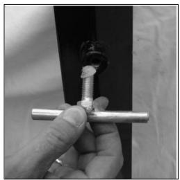
19. Push the saw head up and down the track system to ensure that the width of the track allows for the saw head to move freely. If it binds, the "L" rails will need to be set further or closer together to achieve a consistent width along the entire track system. Once the desired width is achieved, all nuts and bolts can be tightened to the log bunks.
