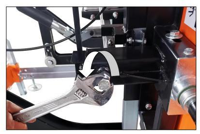
Once satisfied with the measurement, tighten the locking nut clockwise.
