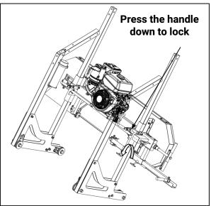
7.With one person on each post, stand the head assembly up on the wheels as shown above. Again, using a minimum of two people, set the saw head assembly on the track system ensuring the carriage wheel grooves rest on the "L" rails. The square vertical post should be on the same side as the log supports
