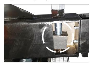
Tracking adjustment bolt out of recess, of it looks like this DO NOT start the mill until it is resting back in its recess
