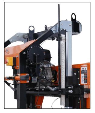
It is important to alternate tightening of the nuts (top then bottom) to ensure the black round clamp begins to compress evenly on both the top and bottom until flanges meet at outer edge.
