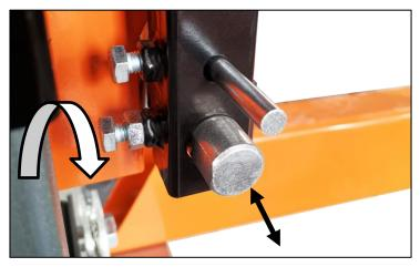
Loosen the blade guide assembly bolt with a socket. The round shaft should now be free to slide rearward and out of the way. Perform this step on both guide assemblies. This will ensure that the guide bearings do not influence tracking of the blade while adjusting.
