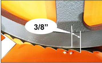
Wearing gloves, spin the bandwheel with your hand and observe how the blade has changed tracking. Measure the distance again and repeat the above step to further compensate if required. The ideal measurement is 3/8".
