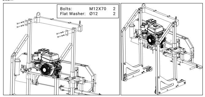
9.Install the connecting clamping plate, uper arch and steel cable roller, using wrench to hold the nut, tighten the bolt
