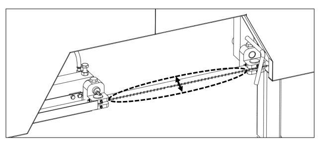
Proper blade tension is achieved when the blade deflects no more than a total of 1/8" - 1/4" up/down when it is firmly moved by hand at the center location of the blade guide blocks. Turning the blade tension "T" handle in the clockwise direction will add tension to blade.
