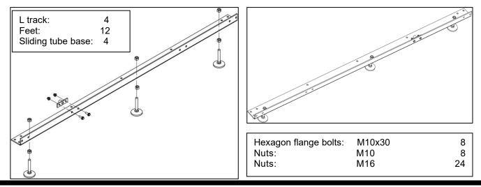
2.Attach track cross supports to "L" channel with the provided nuts & bolts. The joining plate is used at the seam joint to join the two sections together (shown in right-down image). Ensure to only hand tighten at this stage. The bolts will be fully tightened once the head assembly is free to roll on the tracks and provide the correct track width.
