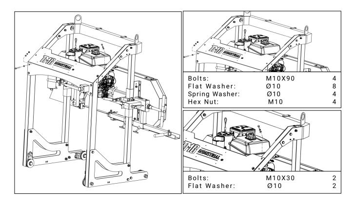
10.Install the lifting system, using wrench to hold the nut ,tighten the bolt.
