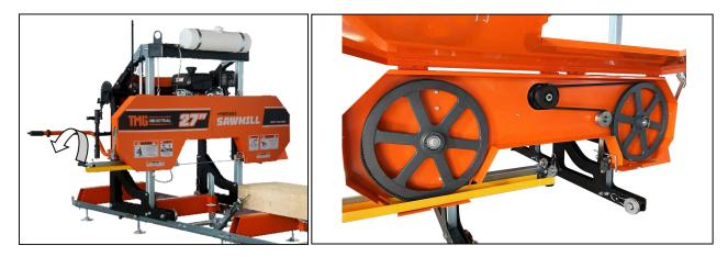
Remove the tension in the blade by turning the "T" handle in the counter-clockwise direction and then open the blade guard cover. The blade should now be loose and free to pull straight out the front. The new blade can now be installed, guards closed and proper blade tension set.
