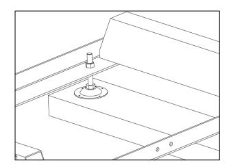
We recommend tex screwing the leveling legs to sleepers once the mill has been made level. So <u>before</u> tex screwing the mill to the sleepers, it is highly recommended that you run a string line down *both* sides of the mill, to make sure the track is straight and level. (The string line is in pink in the above picture).
