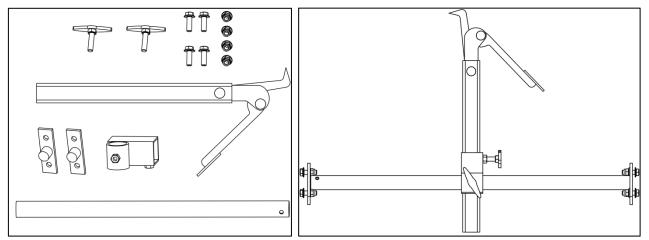
Attach assembly to the track using the provided nuts & bolts and tighten. Attach log dog assembly to track as shown below with the 4 nuts and bolts provided. Note that there are various locations along the track where this assembly can be bolted. Depending on how many track sections are being used, select a log clamp position that will secure the log firmly against the log supports.
