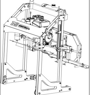
14.Install the travel locking device on the travel assembly, using wrench to hold the nut , tighten the bolt.
