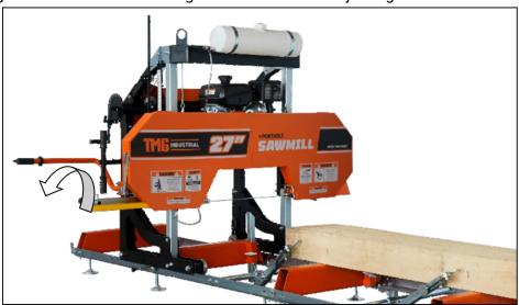
Take some tension off of the blade by turning the "T" handle in the counter-clockwise direction one full turn from full tension position.
