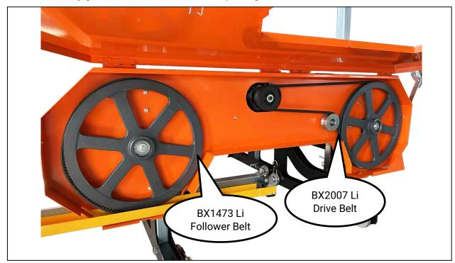
There are two rubber "V" belts on the sawmill and they should be replaced as a set. It is not advised to replace individual belts separately. It is recommended to use a BX2007 Li drive belt for the drive side and a BX1473 Li follower belt.
