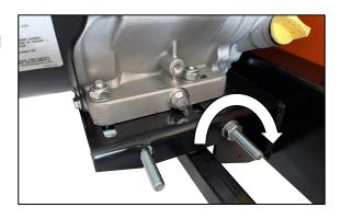
Once the desired belt tension is set, tighten the four engine bolts. *Alternatively, if the drive belt is too tight, the 16mm nut on the horizontal stud can be turned counter-clockwise.*
