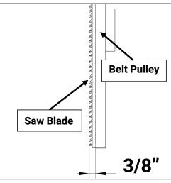
The blade should run with the same tooth to bandwheel face distance on both sides. 3/8" is ideal. Measure the distance from the tip of the blade tooth to the front face of the bandwheel on both sides. If an adjustment on either side is required, the below steps will detail this procedure.
