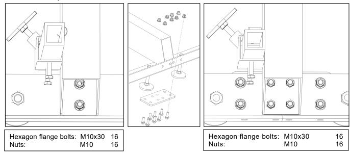
3. Assemble carriage stops at the ends of the tracks (4 stops total) and tighten.
