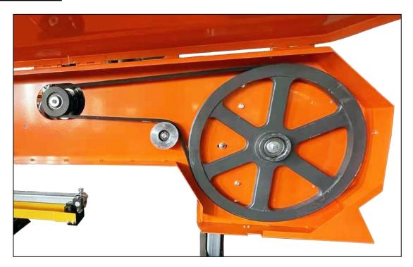
To check the belt tension, with your hand, firmly try to deflect the belt up and down. There should be no more than 1/4" of deflection in both directions (1/2" total). If the belt deflects more than this, it will need to be tightened as described below.
