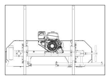
4.Assemble front vertical post to wheel assembly using the two bolts and back plate. Repeat same step for the other front vertical post assembly.
