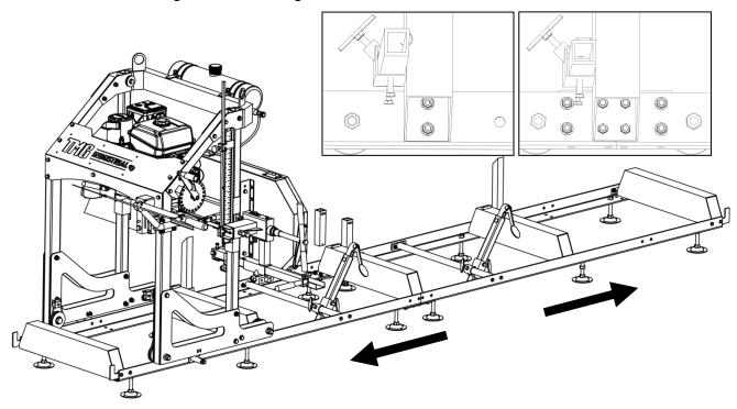
20.Using a tape measure, take a measurement from the blade to the top of the log bunk on both the left and right side. The distance should be equal on both sides. If it isn't, you will need to adjust the cable ends at the rear handle to either raise or lower one side.
