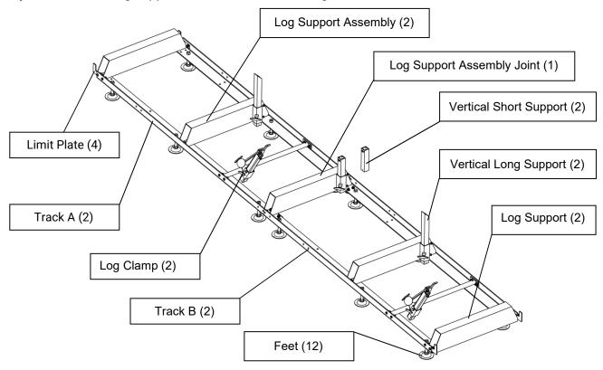
1.Install leveling feet and fasteners to the track, and install the sliding tube base on the track,repeat the above installation until all four are complete
