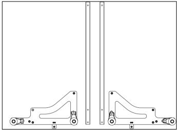
3. Then Insert vertical post assemblies into corresponding locations in head assembly.
