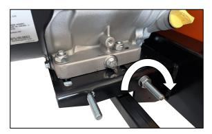
Alternatively, if the drive belt is too tight, the 16mm nut on the horizontal stud can be turned counter-clockwise.
