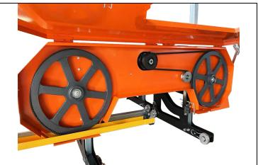
Remove the tension in the blade by turning the "T" handle in the counter-clockwise direction and then open the blade guard cover. The blade should now be loose and free to pull straight out the front. The new blade can now be installed, guards closed and proper blade tension set.
