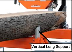
Always cut in the direction shown above. The log clamp should always be on the right side of the log and the log supports should always be on the left. Failure to cut in this direction can cause the log to come lose and possibly even cause damage or injury.
