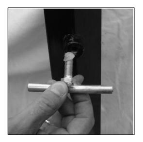
18. Push the saw head up and down the track system to ensure that the width of the track allows for the saw head to move freely. If it binds, the "L" rails will need to be set further or closer together to achieve a consistent width along the entire track system. Once the desired width is achieved, all nuts and bolts can be tightened to the log bunks.
