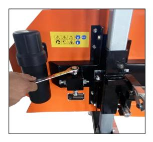
To adjust the left side of the sawmill, again start by taking the tension off of the blade by turning the "T" handle one turn in the counter-clockwise direction. Using a 16mm wrench, loosen the "vertical nut" a ½ turn. Do the same on the "bottom vertical nut". Next, loosen both "vertical bolts" a ½ turn. This will take the clamping force off of the bandwheel shaft caused by these two bolts and allow it to move freely in the following steps.
