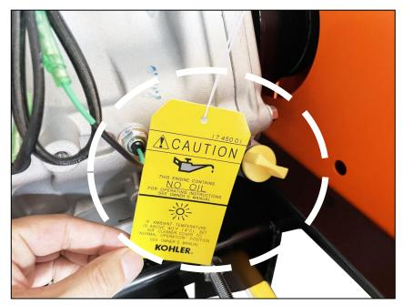
Refer to the engine manual before using your sawmill. Please note that the engine does not contain any petrol or engine oil when it is shipped. Furthermore, the engine is equipped with an oil alert system, meaning that if the crankcase oil level is low or empty, the power is cut to the spark plug and it will not start.
