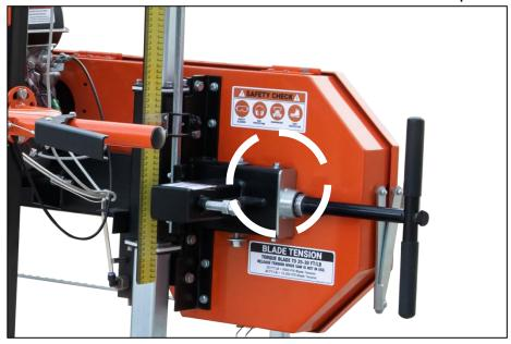
\*Note – It is very important to take the tension off of the blade by turning the "T" handle in the counter-clockwise direction when the sawmill is not in use. Failure to do so, will result in flat spots on the rubber belts. These flat spots will cause the mill to vibrate excessively during next use.\*
