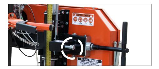
When tensioning the blade, make sure the tracking adjustment bolt sitting behind the T handle (pictured) is sitting back in its recess after you have finished and *before* the mill is run. Failure to do this will result in the blade being thrown and possibly broken.
