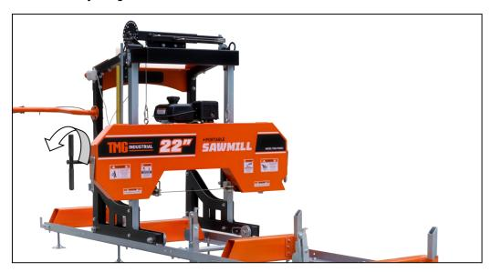
Take some tension off of the blade by turning the "T" handle in the counter-clockwise direction one full turn from full tension position.
