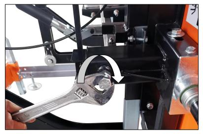
The alignment bolt can now be turned to change the angle of the bandwheel and track the blade. To move the blade more rearward on the bandwheel, this bolt will need to be turned clockwise.
