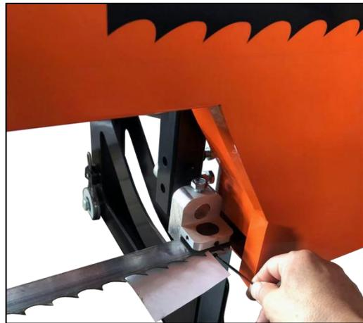
Using a piece of paper in between the blade and blade guide blocks, tighten the allen key bolts.
