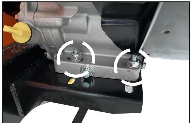
To change the drive side belt, loosen the four bolts that secure the engine to the engine mount using a 16mm wrench.
