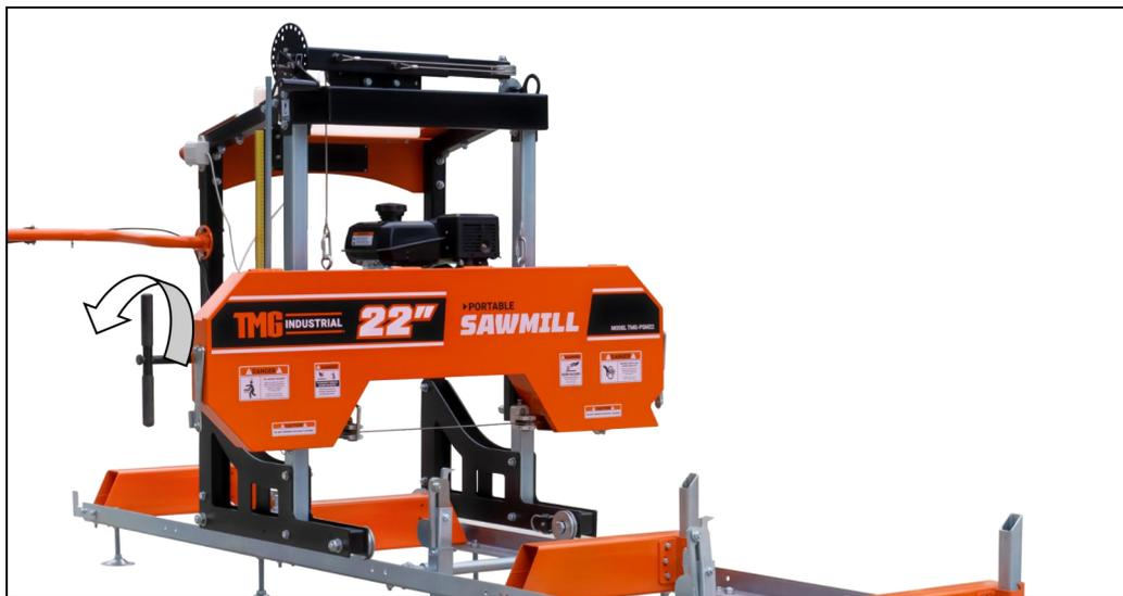
Take some tension off of the blade by turning the "T" handle in the counter-clockwise direction one full turn from full tension position.
