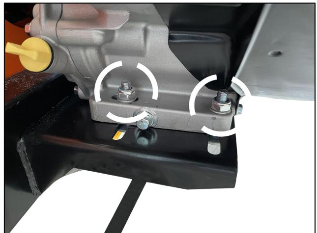
To tighten the drive belt, start by loosening the four bolts that secure the engine to the engine mount using a 16mm wrench.
