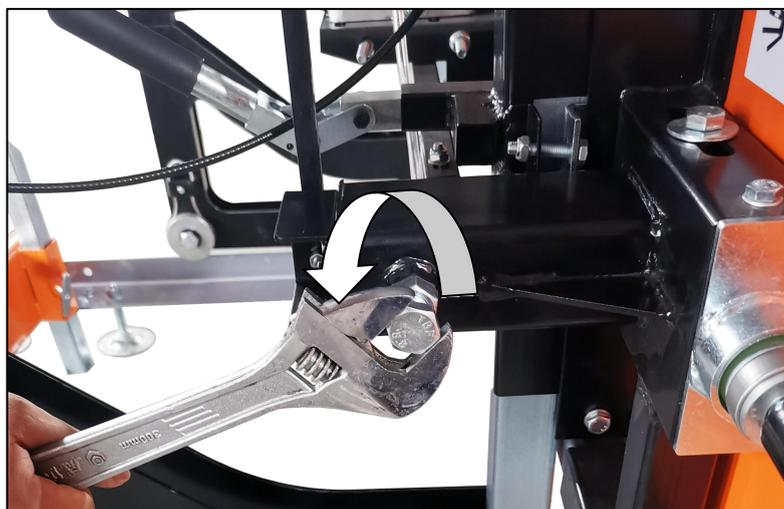
Loosen the tracking alignment locking nut with an adjustable wrench.
