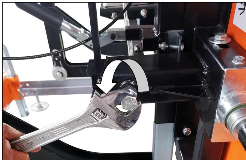
Once satisfied with the measurement, tighten the locking nut clockwise.
