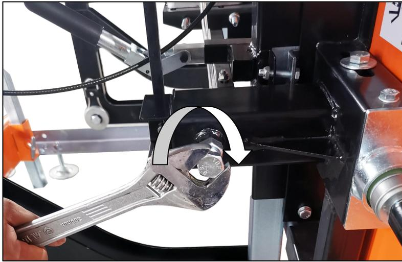
The alignment bolt can now be turned to change the angle of the bandwheel and track the blade. To move the blade more rearward on the bandwheel, this bolt will need to be turned clockwise.
