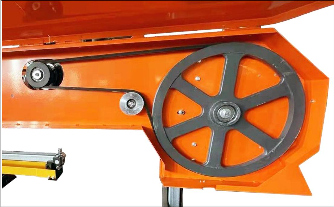
To check the belt tension, with your hand, firmly try to deflect the belt up and down. There should be no more than 1/4" of deflection in both directions (1/2" total). If the belt deflects more than this, it will need to be tightened as described below.
