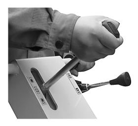
The machine vibratory is controlled by centrifugal clutch. It does not work when the motor rotate speed is low.
