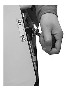
Turn the choke level to the "CLOSE" position.
