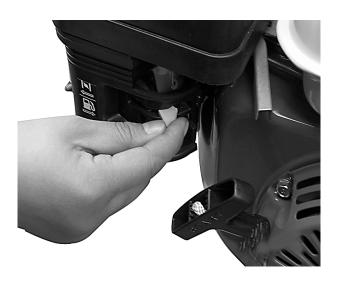
Turn the fuel valve to the "ON" position. Turn the engine switch to the "ON" position.
