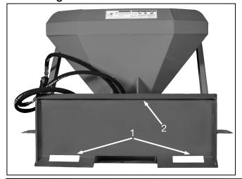
Inspect the heavy duty spreader's mounting flange (1) and wedge mounts (2) [See left photo]. Inspect all welds on the heavy duty spreader for wear or damage each time the heavy duty spreader is removed from the machine.
