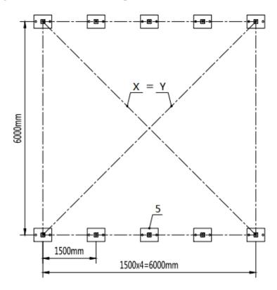
• Installation diagram of expansion bolt.
