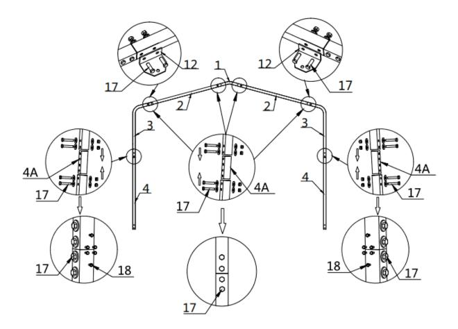
Note : use (#18) at the links of (#3) and (#4) to reinforce the inner side.
