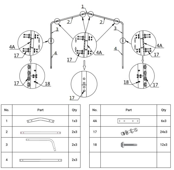
• Lay down all (5) trusses on the ground as figure when the assembly is all completed and before moving to next step.
