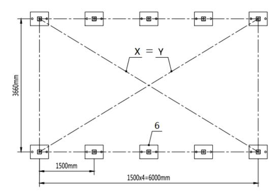
• Installation diagram of expansion bolt.
