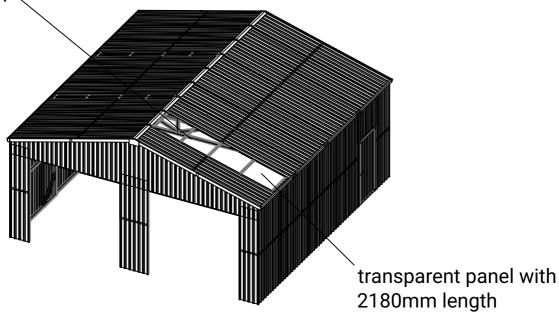
The blank space is where the transparent panels are installed. Please install them according to the correct position. The two transparent panels are stacked together. Incorrect installation will cause water leakage. Please pay special attention.
