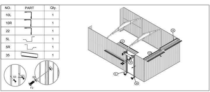
The below assembly is for the front door & roof , pls ignore the side door direction in the assembly picture.
