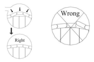
After the top piece is correctly installed, fix the remaining staves with 4\*40mm screws.
