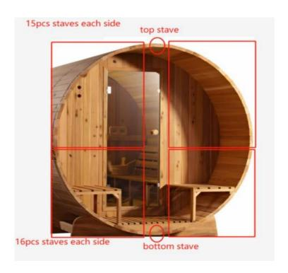
9. The remaining gap will be filled with the 'Top Final Stave' which is available in two sizes. Due to natural swelling/shrinking of the cedar wood, one piece is likely to fit better than the other. Choose the one that fits best.
