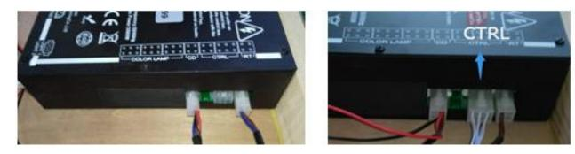
3. Check if all connections to the control box are secure.
