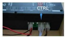
3. Check if all connections to the control box are secure.
