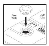
Gas Engine - Gasoline level - The engine is a 4 cycle and uses regular octane, unleaded fuel. DO NOT USE MIXED FUEL. Refer to the engine operation manual included with your pressure-washing unit.
