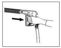
**8.To stop Burner operation** – Turn BURNER switch to 'HEATING OFF' and run pump for two minutes with trigger gun pulled to allow coil to cool down. After cooling period is complete, turn off main power to motor by turning BURNER switch to 'OFF' (turn PUMP switch to 'OFF' if equipped with auto start stop). Squeeze and release the trigger for the second time in order to relieve the pump system of pressure.
