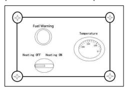
IF YOU EXPERIENCE IGNITION FAILURE, DO NOT ATTEMPT TO RESTART BURNER! EXCESS FUEL AND VAPORS MAY HAVE ACCUMULATED AND THE CHAMBER MAY BE HOT. THE UNIT MUST COOL DOWN BEFORE RESTART CAN BE ATTEMPTED.
