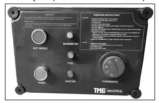
IF YOU EXPERIENCE IGNITION FAILURE, DO NOT ATTEMPT TO RESTART BURNER! EXCESS FUEL AND VAPORS MAY HAVE ACCUMULATED AND THE CHAMBER MAY BE HOT. THE UNIT MUST COOL DOWN BEFORE RESTART CAN BE ATTEMPTED.
