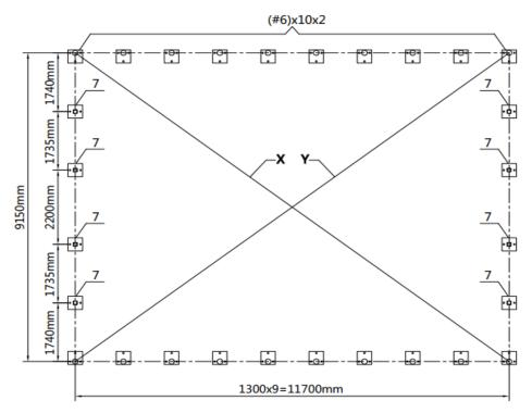
• Installation diagram of expansion bolt.
