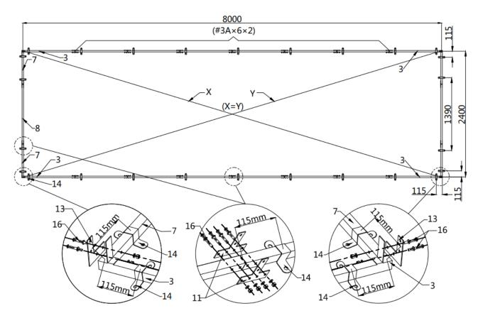
• Installation diagram of expansion bolt.
