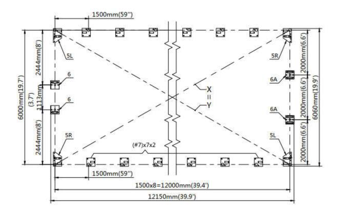
· Installation diagram of expansion bolt.
