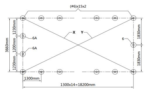
• Installation diagram of expansion bolt.
