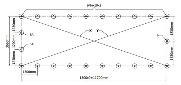
• Installation diagram of expansion bolt.
