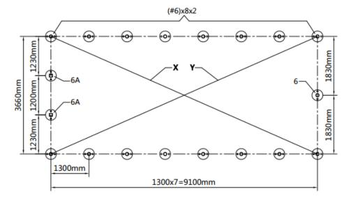
Installation diagram of expansion bolt.
